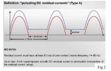
**Type A RCCB** / *EN61008-1* Suitable for use with AC and pulsating DC with a maximum DC content of <6mA (Fig 1). If more than 6 mA DC flows through the RCCB, the tripping characteristic will be altered due to the saturation effect of the DC current on the A Type sensing coil. As the level of DC current increases the tripping time will increase to a point where the coil is completely saturated and the RCCB will not operate *– see clause 133.1.3 IEE Wiring Regulations*.
