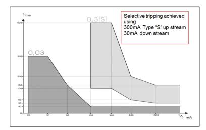
To achieve full discrimination with a 30mA device, the upstream RCD must be at least 300 mA Selective. i.e. the characteristics of the devices do not overlap at any point in the diagram opposite. Using a 100mA with 30mA device could result in both devices tripping under certain fault conditions. Selective RCDs are available in Type AC, A and B versions.
