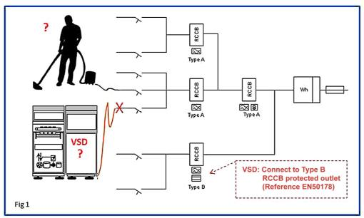
If the RCD cannot detect the leakage current e.g. outside of the designed frequency range, or the magnetic circuit is saturated (dc superimposed on the ac wave form) it will not trip. Obviously protection will only be maintained if the RCD is working within its original design limits.
