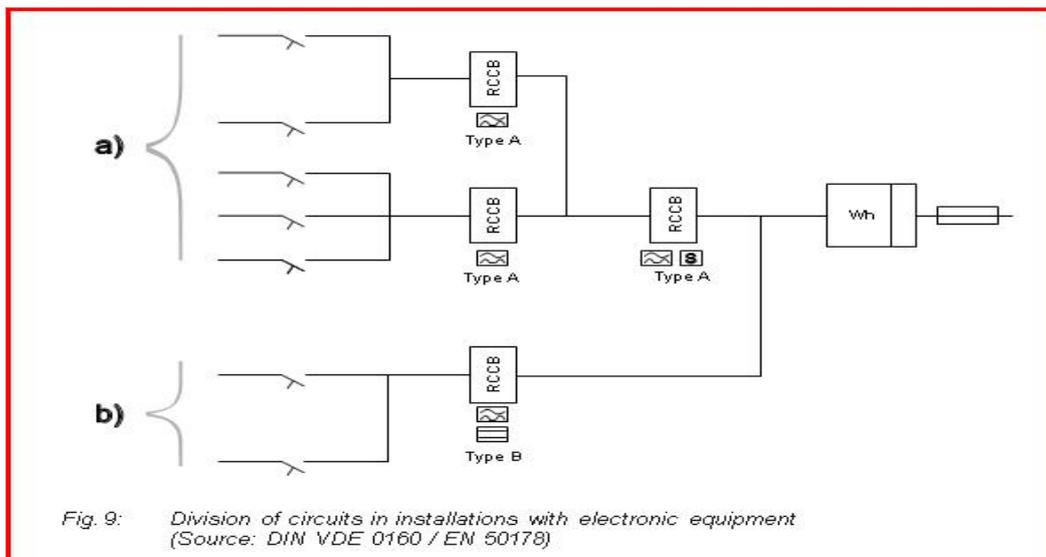
Type B RCCBs are designed to sense DC earth leakage currents as well as high frequency AC leakage currents, which are also generated as a result of PWM and the associated filters (required to meet EMC regulations)– especially within lower cost solutions.
