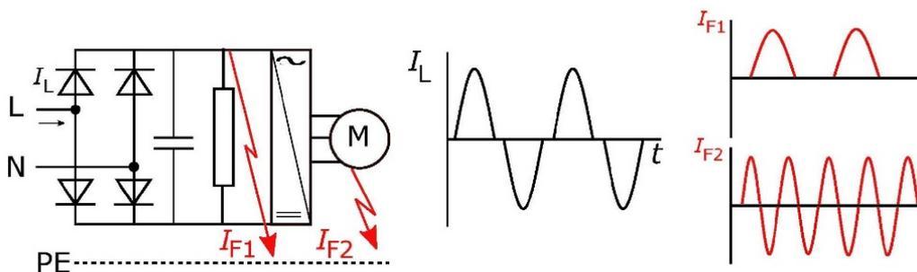
Other common applications using single phase inverters, pumps, tools, battery charging. Mode 3 Charging of certain vehicles may require Type F (IEC60364-7-722 Ed2 Sept. 18 Now makes reference to Type F).
