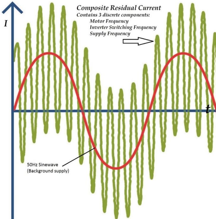
Operational leakage currents and residual currents associated with circuits containing non – linear loads i.e. current drawn is not proportional to the supply voltage, will consist of mixed frequency components creating a composite residual current - see Figure 1.
