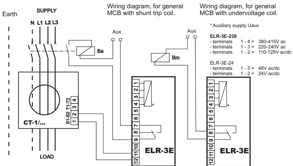
The output contact can be used also for tripped relay signalling only, without connecting the output to the tripping coil.
