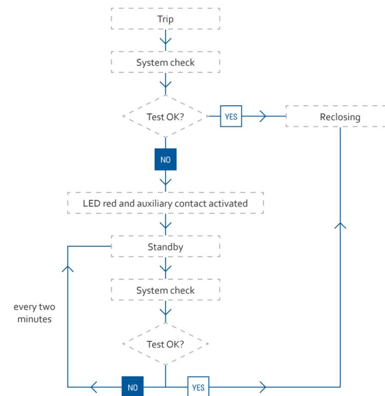
When the 'Selftest Restart' is tripped, a simplified insulation resistance test is performed.
