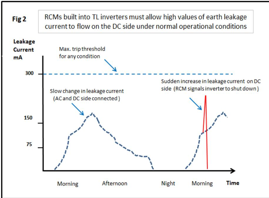
something is creating a low resistance path to earth. In this situation the RCM should feed signals to the control section of the inverter, to indicate a fault condition /sound an alarm and disconnect the AC side of the inverter from the DC side. Disconnection is normally carried out by the same relay contacts used for interface protection with the DNOs distribution system. Don't forget the PV generator is always considered to be energised irrespective of the operational state of the inverter.
